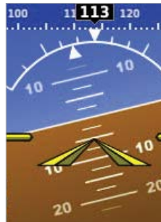
Figure 2-8 Sky Pointer Configuration
